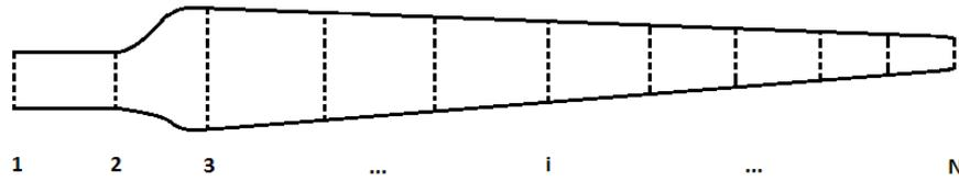
Figure 6.3: Sections along a blade
